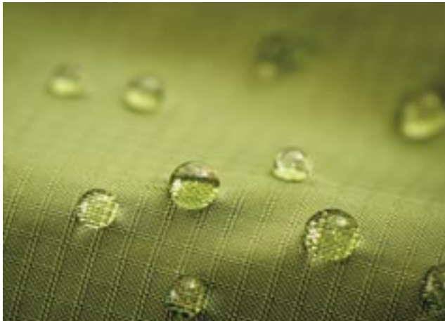
Empel-treated fabrics show a 25% lower uptake of water because of the uniformity of its application to fabric. Encapsulating each of the fibres works better than top-coating. It also avoids the problem of 'bridging' that often occurs with wet-finishing.
